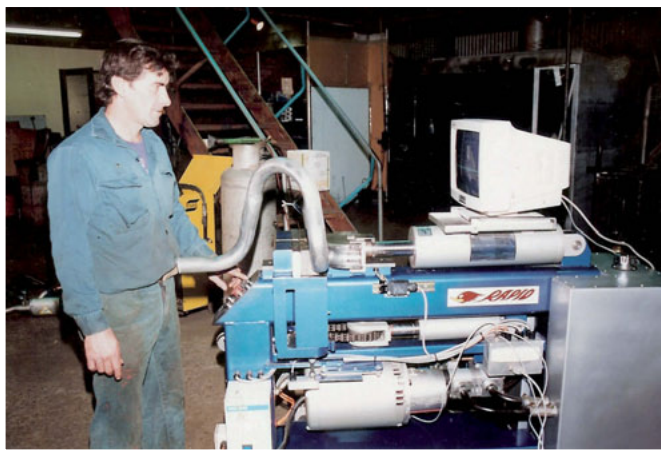
This computer controlled press bender was supplied by Rapid Equipment for Rapid's manufacturing division. Note the large capacity oil pump and tank and the electronic rotation gauge.
