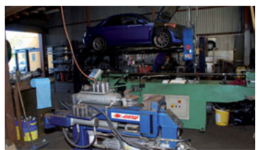
STAGE 1: The development vehicle on the vehicle hoist located in Rapid's manufacturing section and the old exhaust is being removed.
