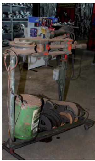
Yes, this exhaust bender does work and served for many years to launch what was probably Australia's first muffler shop. In more recent times it was utilised to bend frames for motorcycle speedway sidecars which were raced by long-time Rapid employee, Terry Gunter. It now serves as a showroom display highlighting the company's heritage.
