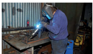
STAGE 6: The flanges, catalytic converters and hangers are welded into the system.
