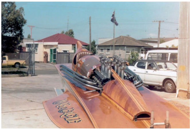
In past years Rapid has been called upon to design and manufacture special exhaust systems such as this example.
