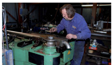
STAGE 3: Bending commences using patterns and checked against measurements.
